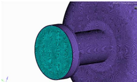
Figure 4: Model of the fluid meshing
